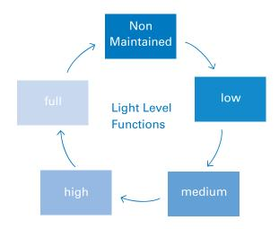
Preset light levels can be adjusted in Maintained mode to operate as security light, adjustable using touch sensitive button on luminaire fascia.
