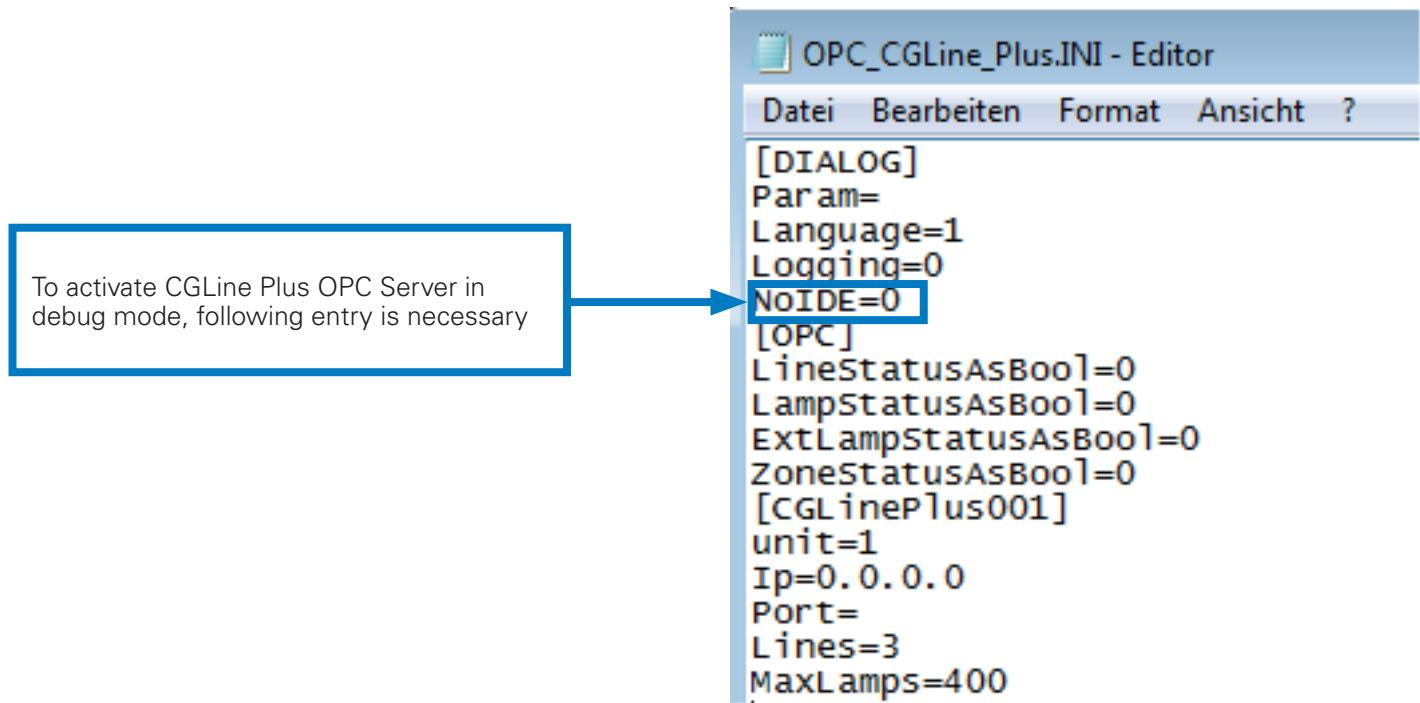
*ATTENTION: Remove the debug mode (set NoIDE=1), when the BMS configuration has finished.*
