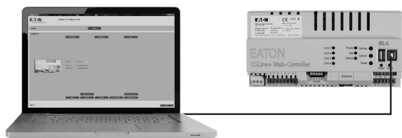
Fig. 3. Connecting the controller to a laptop with CGLine+ PC-Software via USB A-B
