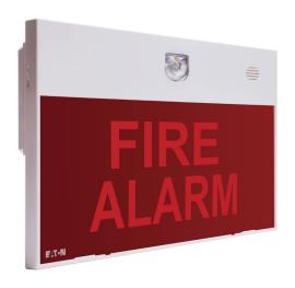
EFSB is a durable sounder/beacon that is certified to EN 54 applicable standards. Boasting impressive aesthetical and durable design, it ensures reliability and energy efficiency. It has been purposely designed for installations where aesthetics plays a key role. The device is supplied with a label carrying the text "FIRE ALARM", LED backlit in case of alarm. Two alarm tones are selectable via jumper: 970Hz / 2500Hz.
