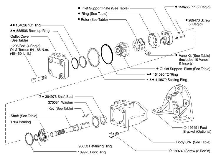
☐ Assemble seal with spring loaded sealing member towards bearing. Seals to be completely wetted with oil prior to assembly.
