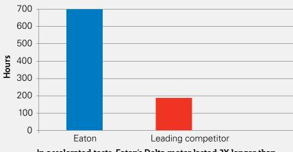
In accelerated tests, Eaton's Delta motor lasted 3X longer than the competition.
