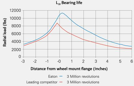
Each curve is based on B 10 bearing life (2000 hours of 12,000,000 shaft revolutions at 100 RPM) at rated output torque.
