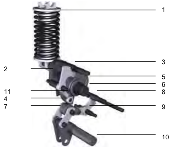
Fig. 6-9: Breaker Closed and Closing Spring Charged
