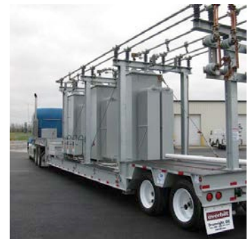
Modular integrated transportable substations
