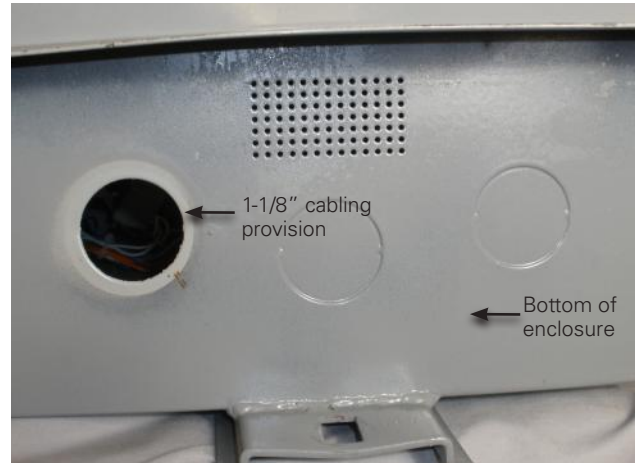
Figure 30. Control enclosure bottom access.
