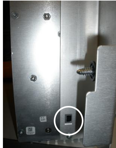
Figure 26. Neutral light source switch.
