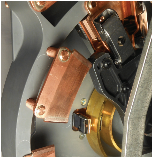
Figure 6. Stationary contact removal and installation.
