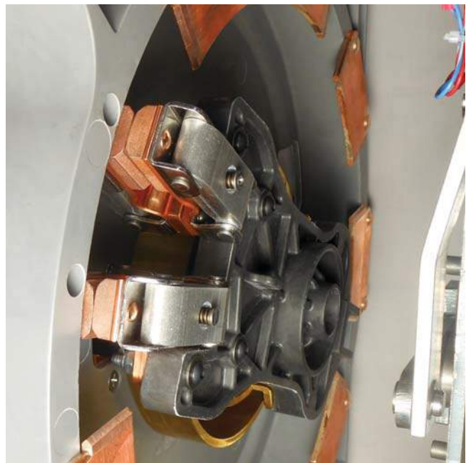
Figure 8. Rotating and removing the movable contact panel assembly
