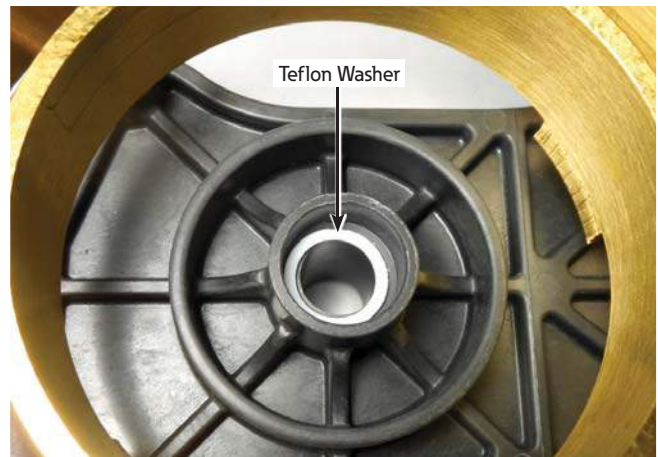
Figure 12. Teflon washer placed in contact panel recess
