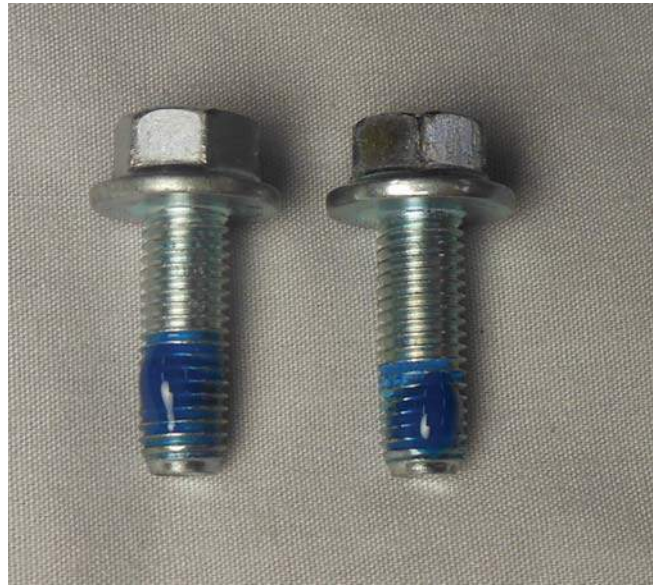
Figure 19. Actuator finger bolts with Loctite® Threadlocker
