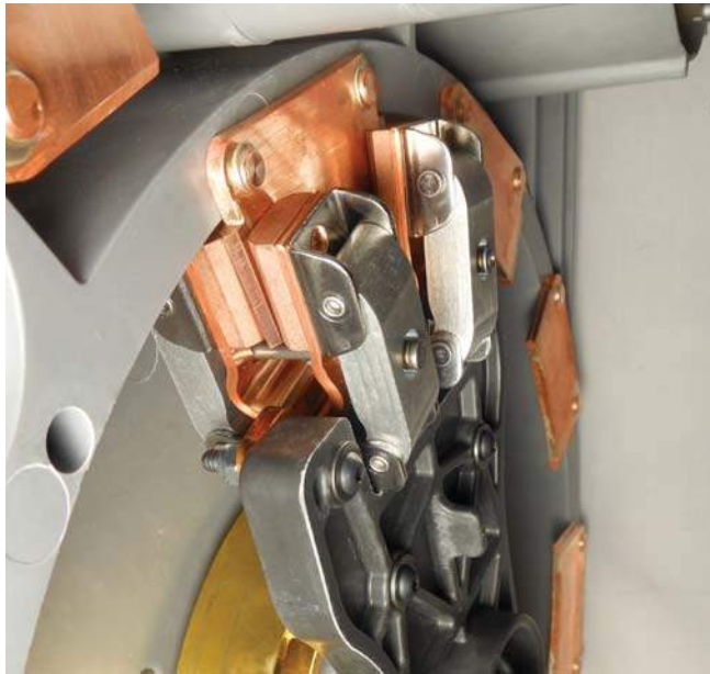
Figure 14. Movable contacts rotates over the neutral stationary contact
