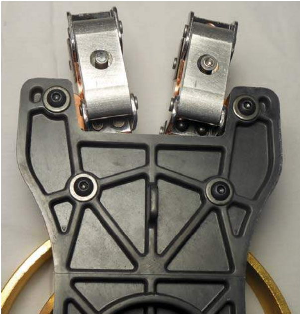
Figure 10. Use 5/32" Allen wrench for screw removal
