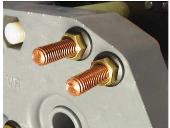
Figure 18. Reinstalling neutral stationary and hardware
