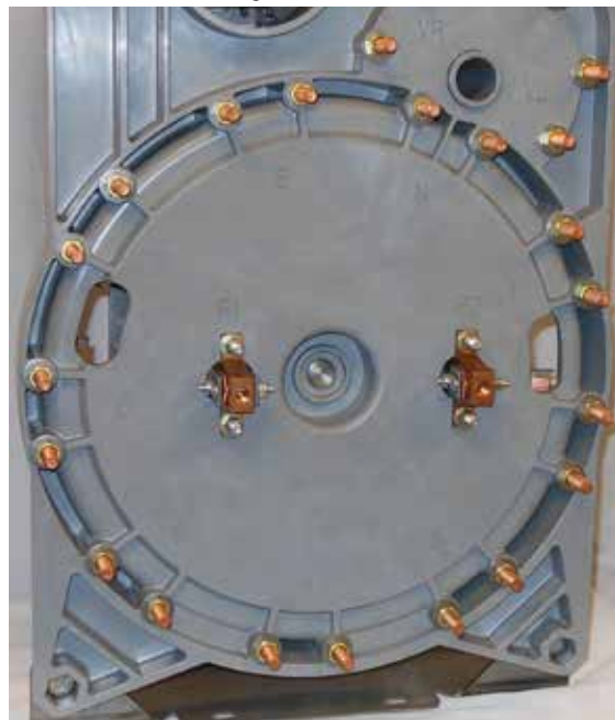
Figure 79. Removal of contact hardware.
