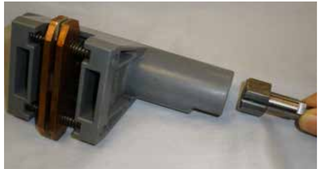
Figure 39. The actuator shaft removed from the reversing movable contact assembly.
