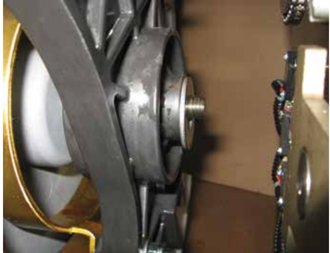
Figure 146. Installing main shaft.
