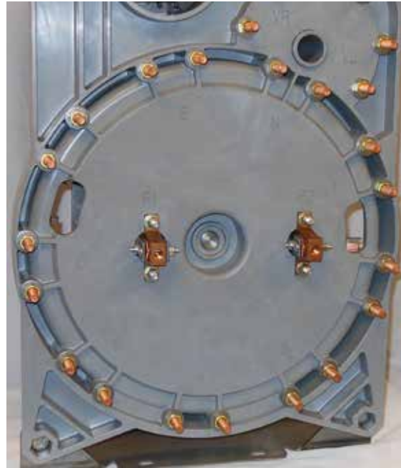
Figure 3. Removal of contact hardware.
