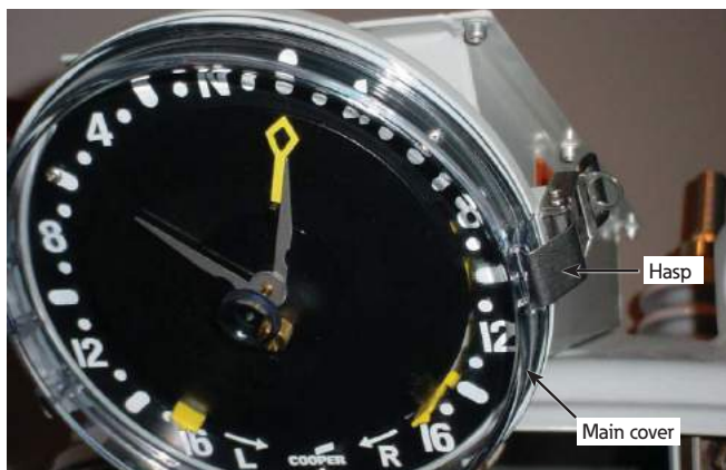
Figure 6. Latching position indicator main cover
