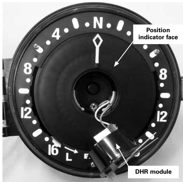
Figure 5. Removing the DHR module
