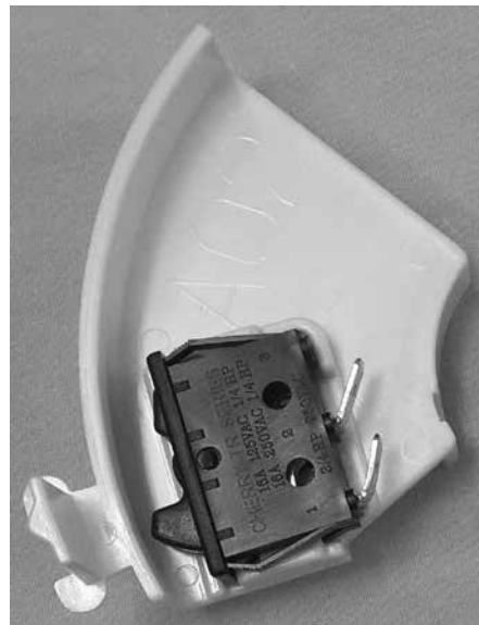
Figure 2. Left-hand/lower limit switch assembly
