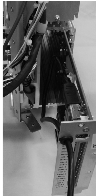
Figure 4. Inserting the I/O module into the accessories slot in a multi-phase control.
