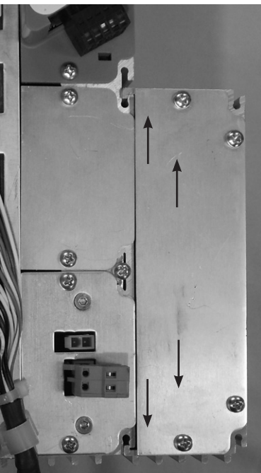
Figure 3. Auxiliary accessory extrusion attached to back of main control. The extrusion may be installed in any one of three locations on the back of a control.
