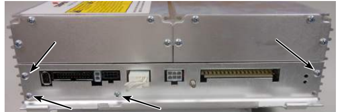
Figure 30. Removal of hinged side panel from CL-7 control
