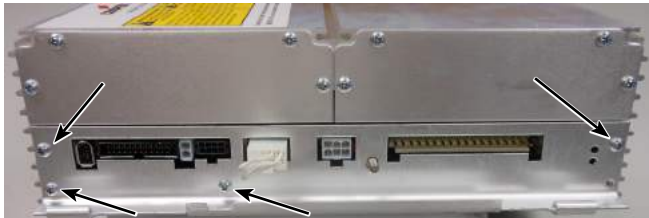
Figure 38. Removal of hinged side panel from CL-7 control
