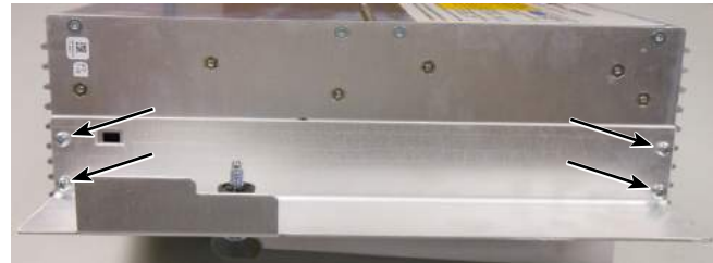
Figure 27. Removal of latch bracket from CL-7 control
