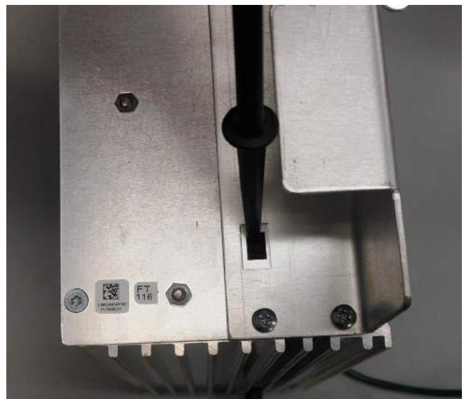
Figure 14. Setting neutral light configuration switch
