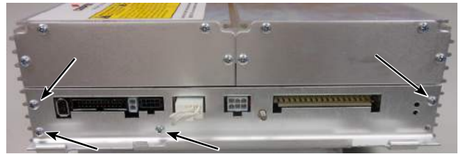
Figure 45. Removal of hinged side panel from CL-7 control
