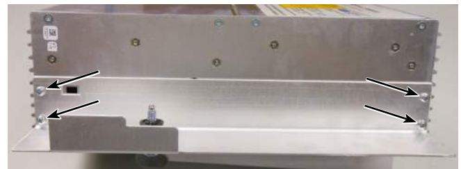
Figure 17. Removal of latch bracket from CL-7 control
