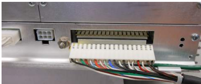
Figure 12. Removal of standard wiring harness
