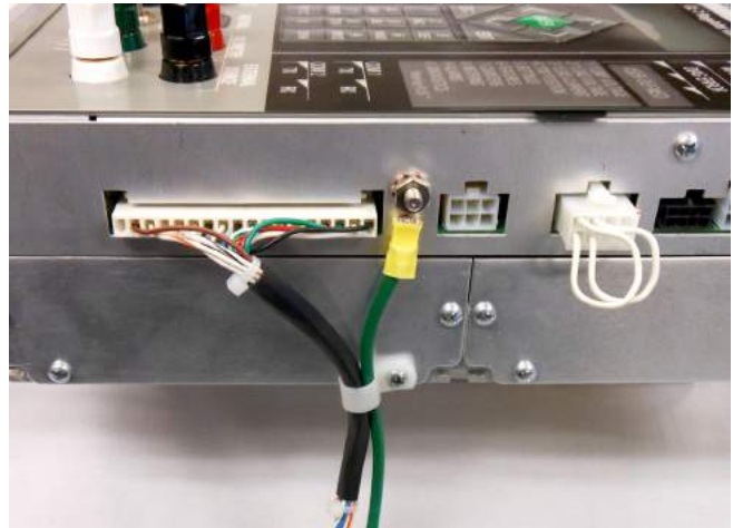
Figure 21. Installing ground wire and Siemens Corporation wiring harness
