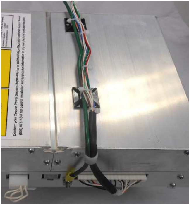
Figure 47. Installing ground wire and harness cable ties
