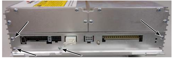
Figure 20. Removal of hinged side panel from CL-7 control
