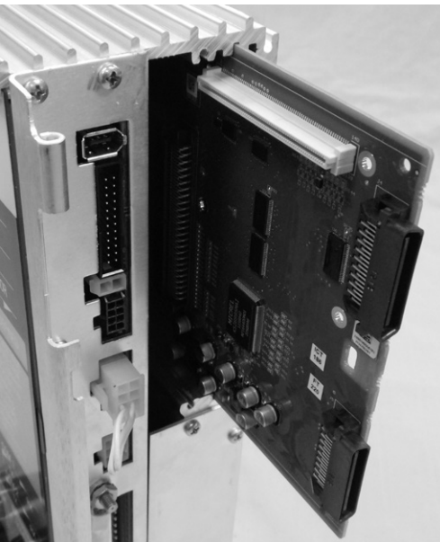
Figure 3. Installing the communications base board
