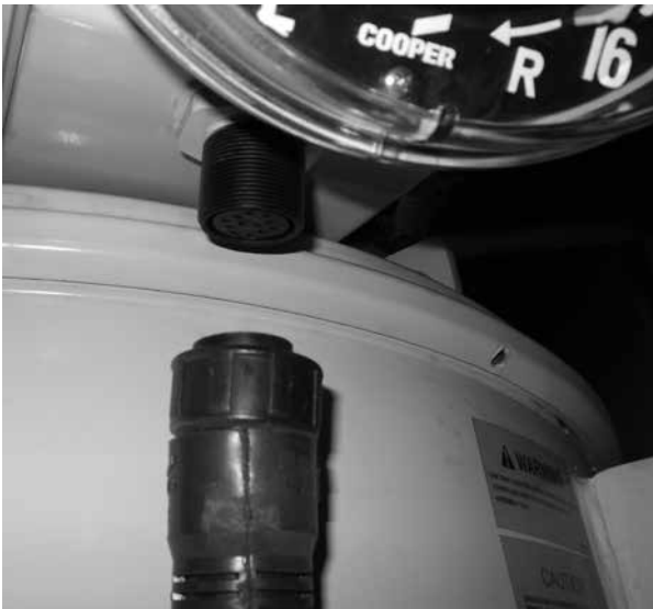
Figure 3. Disconnecting the control cable under the junction box
