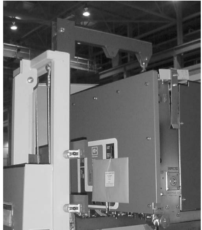
Figure 9. Lifting and Setting the Breaker in the Housing.
