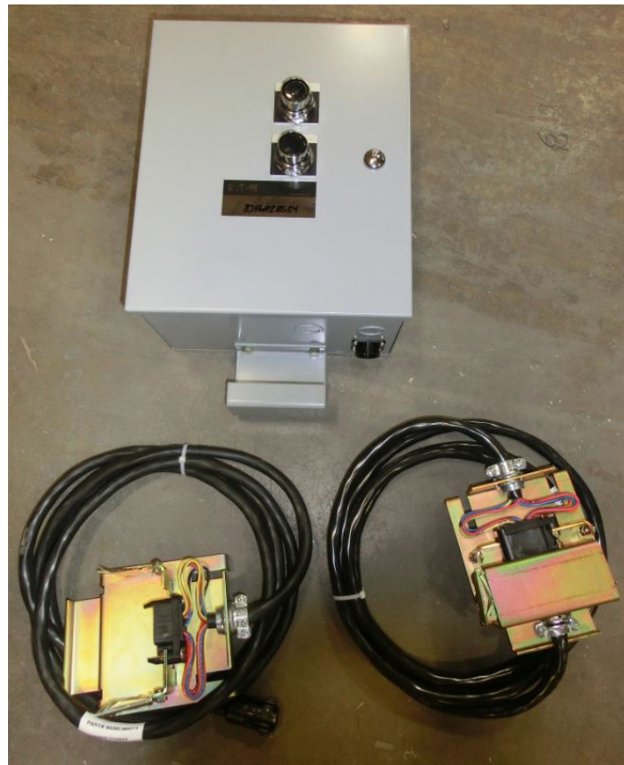
Figure 51. Test Cabinet and Test Jumper.
