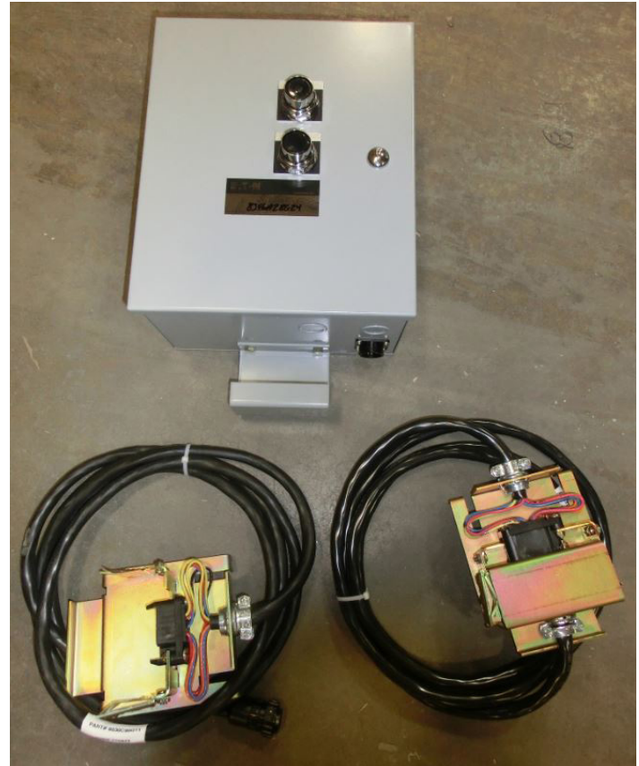
Figure 21. Test Cabinet and Test Jumper.
