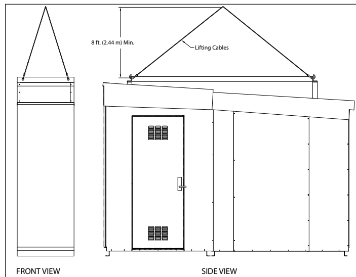
Figure 4. Lifting Angles for Outdoor Sheltered Aisle.
