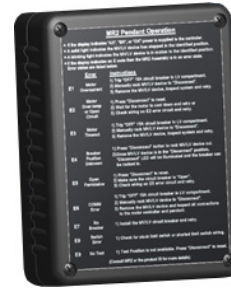
Figure 10. MR2 O/C error code display.
