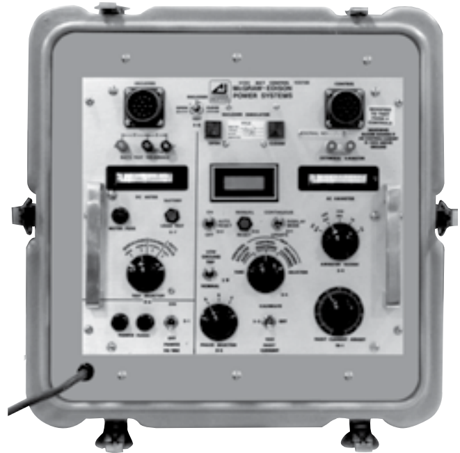
Figure 40. Type MET electronic recloser control tester
