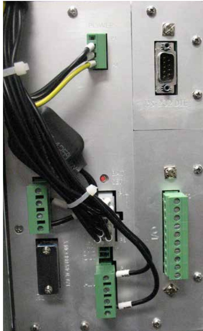
Figure 6. SPEAR single-phase recloser control-side panel communication port.
