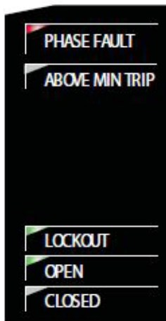
Figure 9. Status Indicator LEDs.
