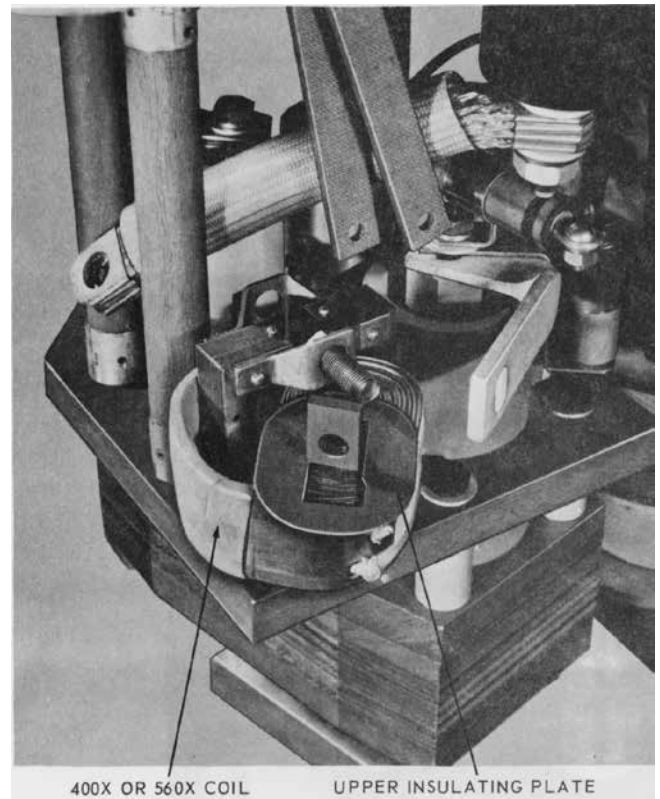
Figure 3. Inserting 400X or 560X series coil into solenoid frame.
