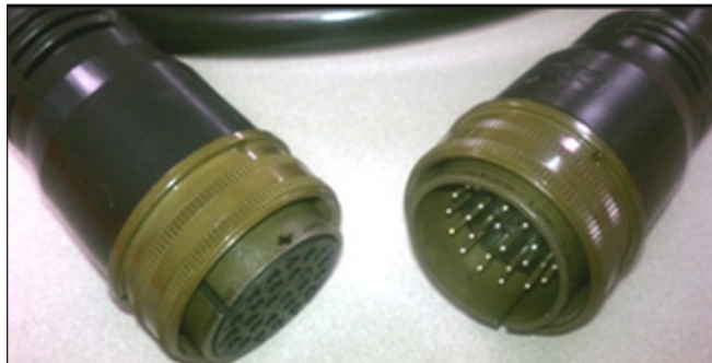
Figure 7. Cable with aluminum cable coupler ring.
