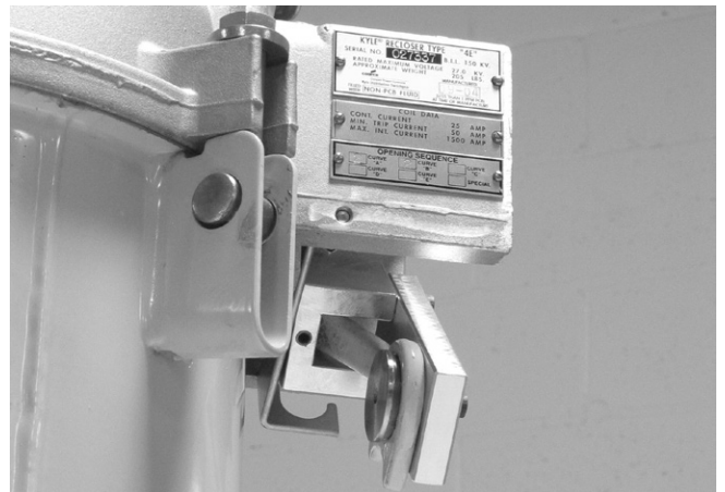
Figure 10. TA10557000 fixture installed upon recloser lever with centering cone passing through ring of recloser operating lever
