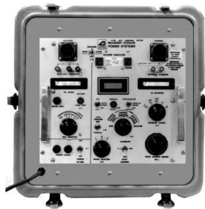
Figure 35. Eaton's Cooper Power series type MET electronic recloser control tester
