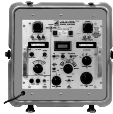
Figure 42. Type MET electronic recloser control tester
