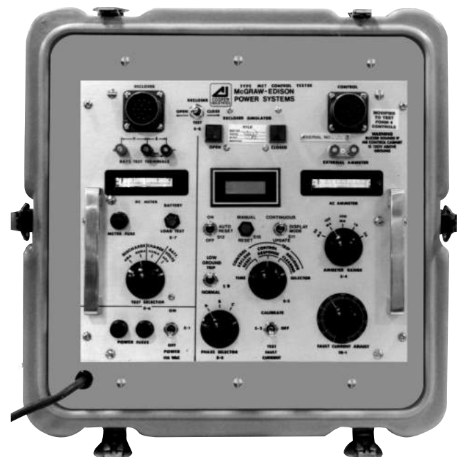
Figure 30. Type MET electronic recloser control tester
