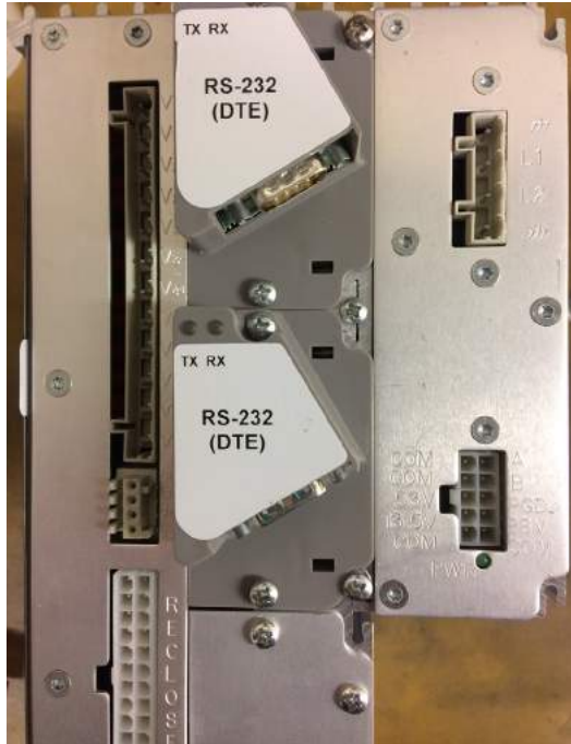
Figure 13. Two communications modules installed
