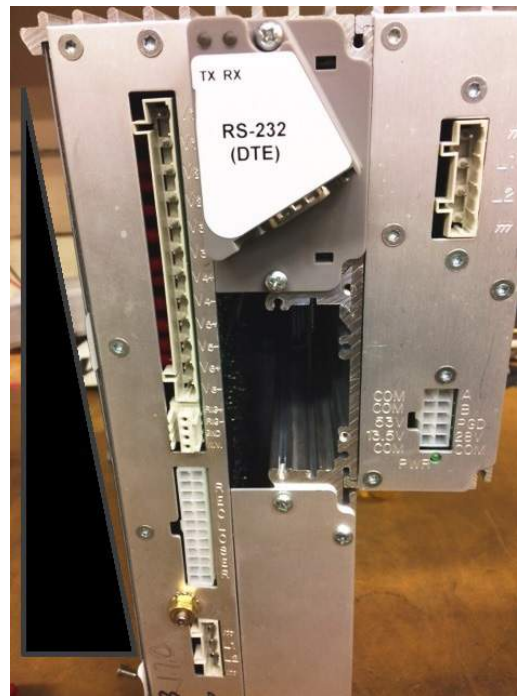
Figure 12. Communications module secured with screws
