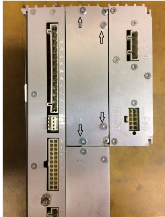
Figure 3. Remove screws shown to open the cover of the communications module slots
