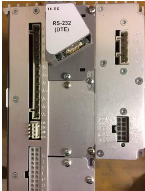
Figure 14. One communications module installed with the other slot covered
