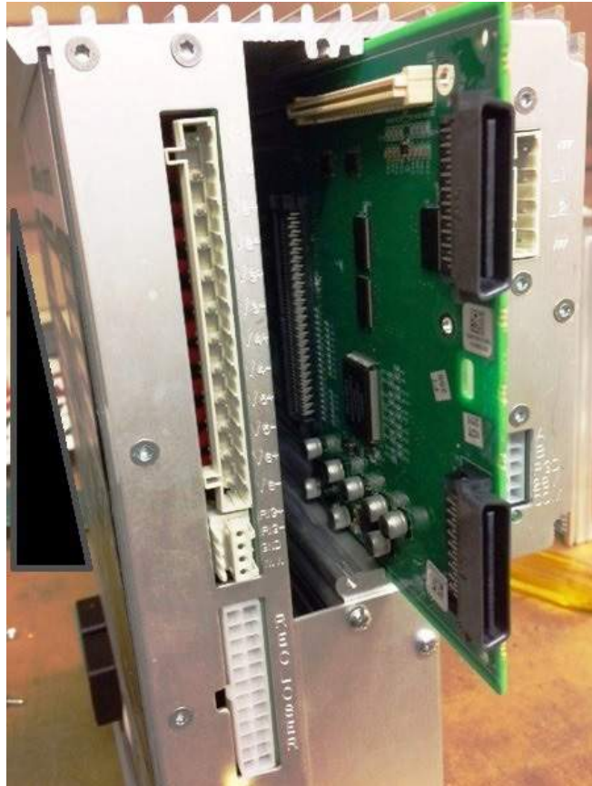
Figure 5. Installing the communications base board
