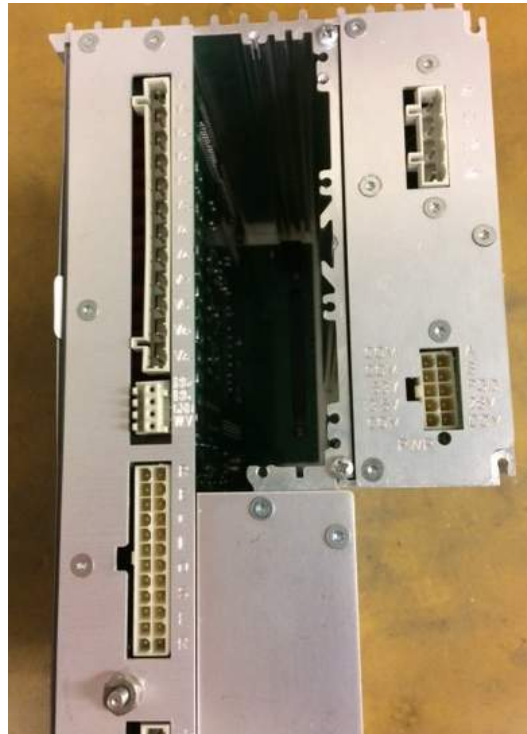
Figure 4. Communications module slots with cover removed
