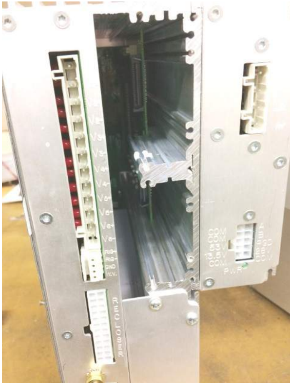
Figure 10. Support bar fully inserted and secured with a screw
