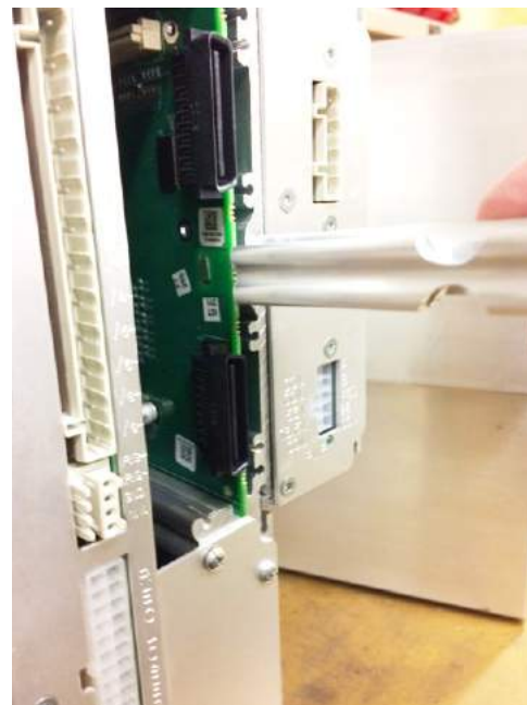
Figure 8. Hooking the support bar nib into the hole in the base circuit board
