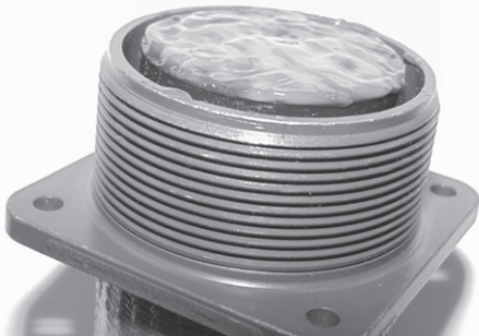
Figure 4. Female receptacle with dielectric grease applied
