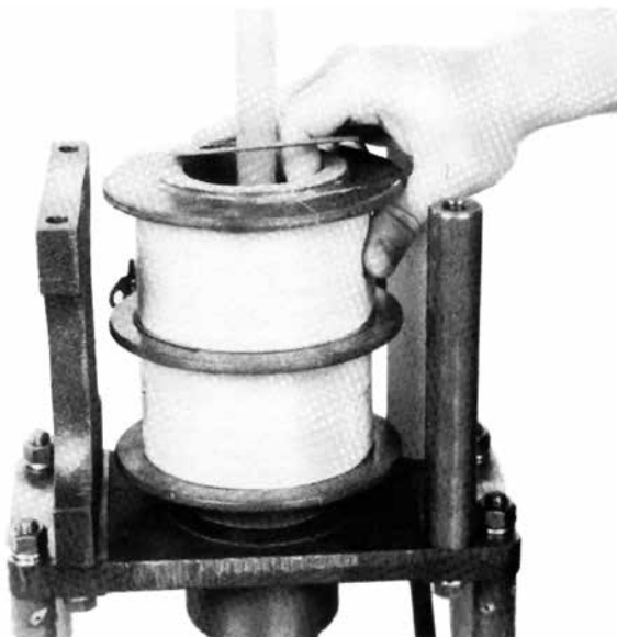
Figure 6. Removing closing coil.
