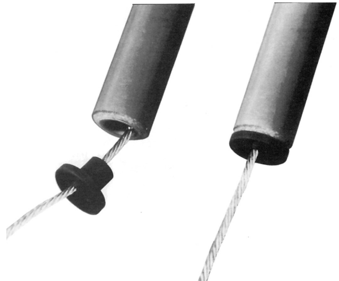
Figure 4A and 4B. Nature Guard expulsion fuse tube plug protects against insect nest building in fuse tubes. Figure 4A shows the plug threaded on the fuse leader and Figure 4B shows final installation.
