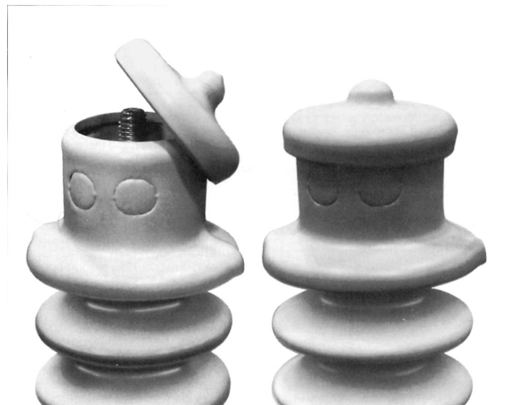
Figure 2A and 2B. Nature Guard CCM31A1 terminal cover showing its two-part construction (Figure 2A) and typical installation (Figure 2B). Note that the lid screws on the threaded bushing stud.
