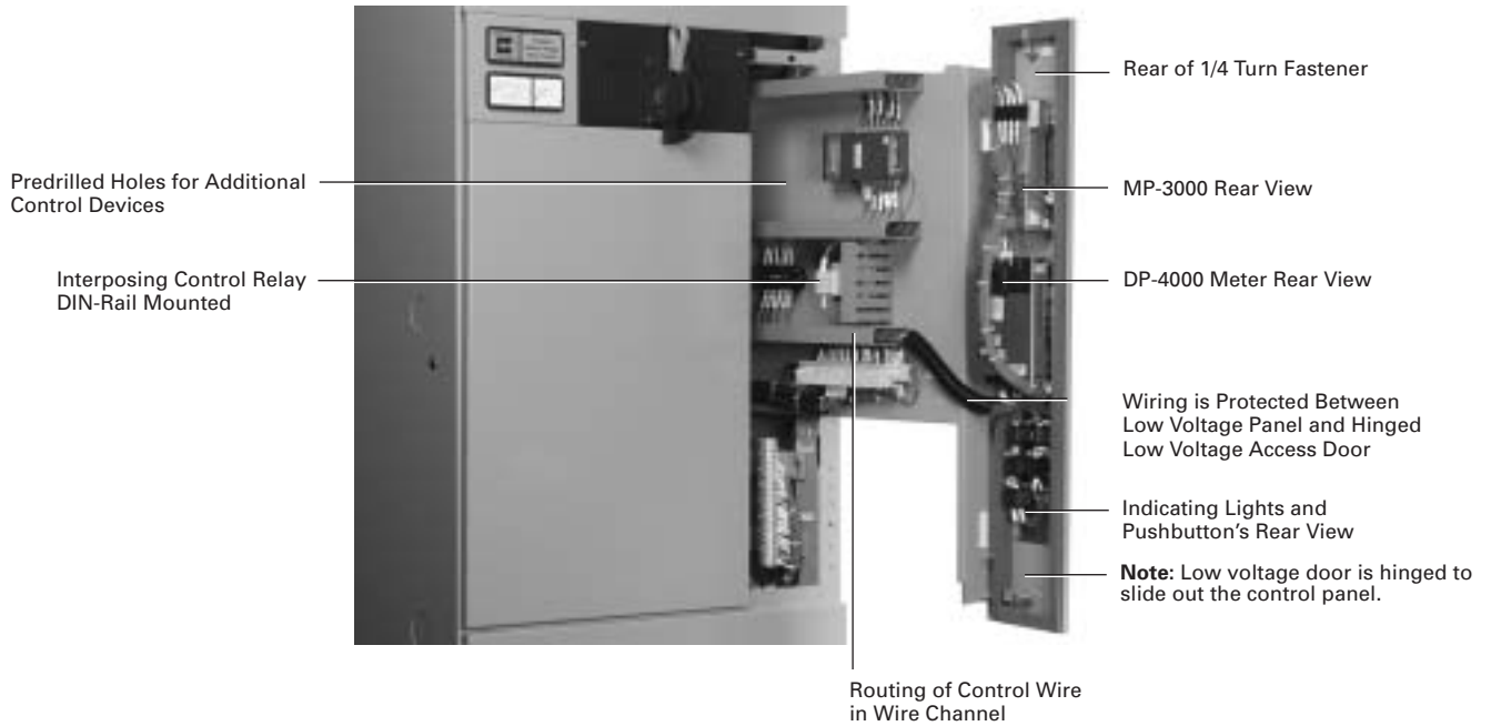
Low Voltage Panel Completely Extended
