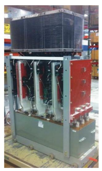
The SC9000 medium voltage drives manufactured from 2007 to 2013 featured potted inverters of which most of the components, including IGBTs, are no longer available due to obsolescence. In the case of a failure, avoid unexpected downtime by taking a proactive approach with one of our two inverter replacement and upgrade solutions.
