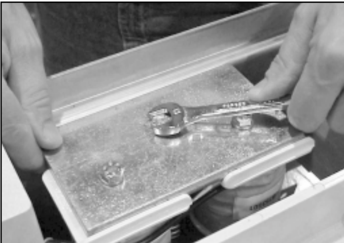
Fig. 29 Remove the locknut securing the return spring bolt
