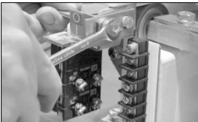
Fig. 32 Remove the two mounting screws securing the contact assembly to bearing retainer
