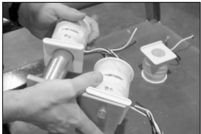
Fig. 31 Install new coils on cores
