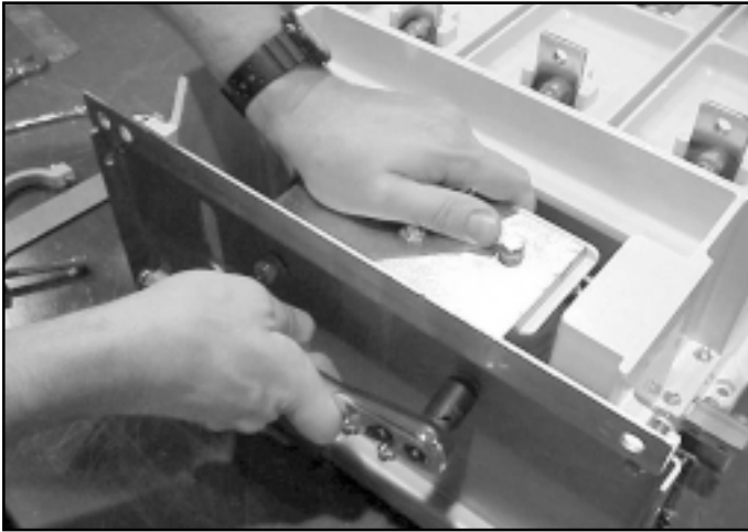
Fig. 28 Remove the coil mounting angle
