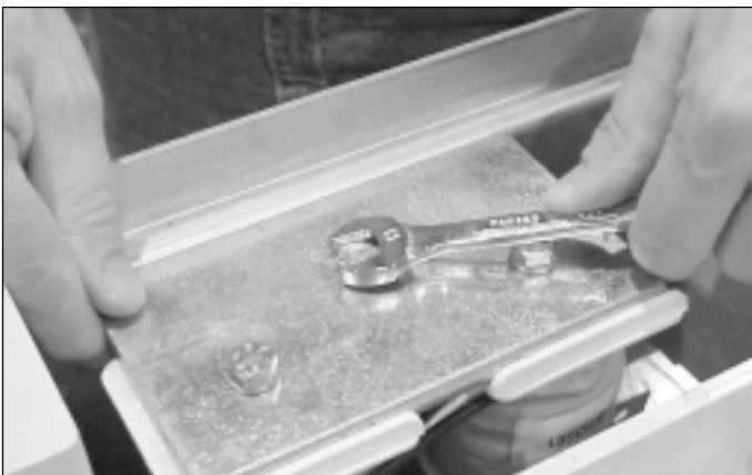
Fig. 27 – Remove the locknut securing the return spring bolt
