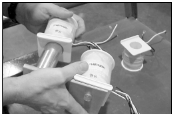
Fig. 29 Install new coils on cores
