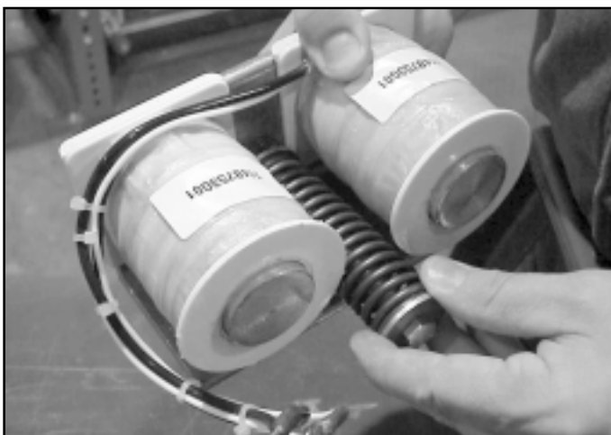
Fig. 28 Unscrew the return spring assembly
