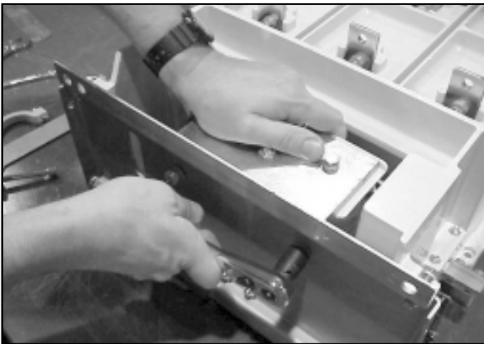
Fig. 26 Remove the coil mounting angle
