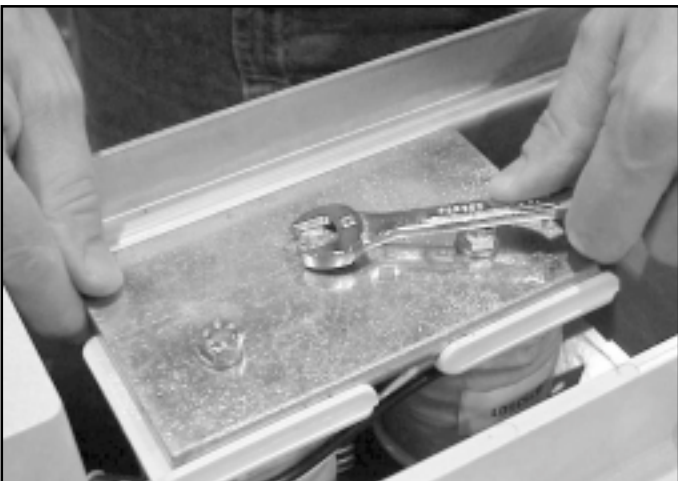
Fig. 27 Remove the locknut securing the return spring bolt
