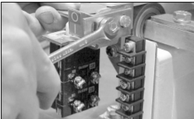
Fig. 30 Remove the two mounting screws securing the contact assembly to bearing retainer
