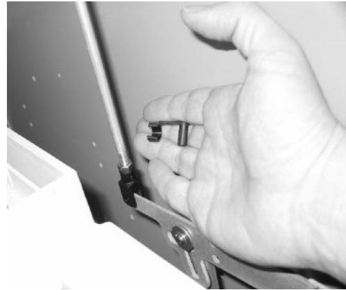
FIGURE 24. REMOVE COLLAR/PIN (PHOTO FROM 400 AMPERE STARTER FOR CLARITY)
