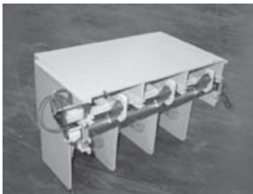
Figure 6. Removable Portion—ISO Switch
