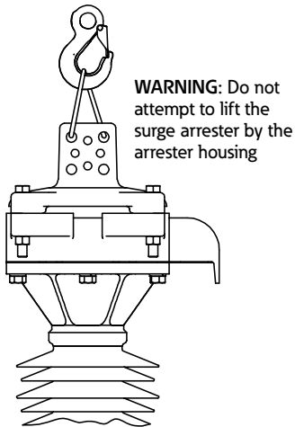
Figure 3. Detail of recommended lifting instructions
