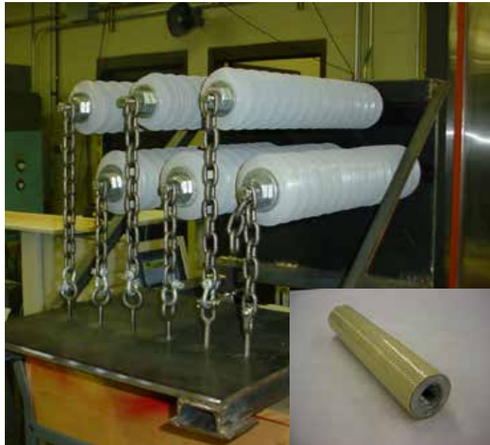
Completion of bending moment test per IEEE C62.11 design
