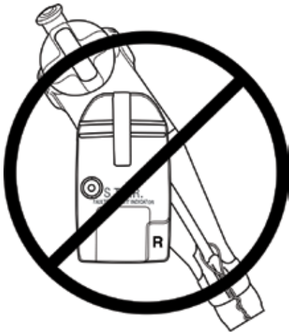
Figure 4. Incorrect methods of aligning Loadbreak elbow with fault indicator
