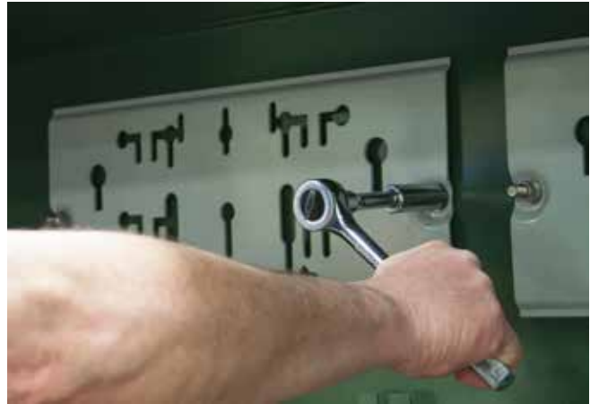
Figure 2. Mounting plate removal.
