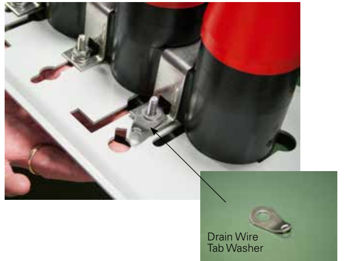
Figure 7. Install drain wire tab washer.
