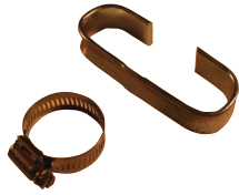
Figure 17. Tie wire assistant
