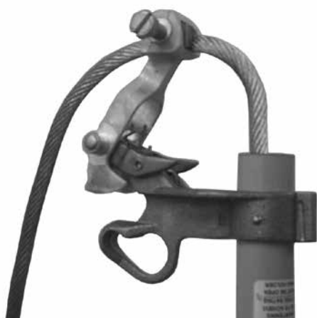
Figure 8. Installing a fuse link in a 200 A fuse holder.
